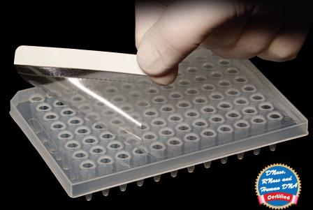
NOVAS BIO offers two approaches to sealing PCR plates using films. Both can be used on 96 and 384 plates.
