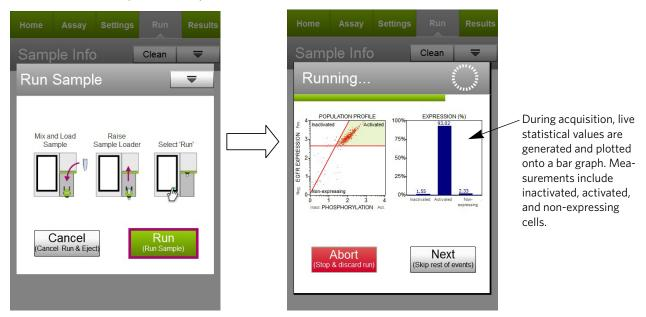
11. When acquisition is complete, the results are displayed. If desired, select **Plots** to display a dot plot and a bar graph for the sample.
