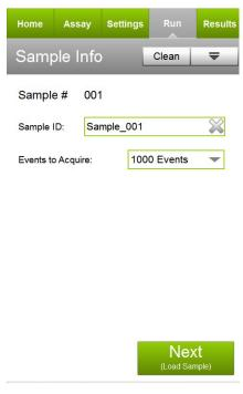
10. Follow the on-screen instructions and mix the first sample. Load the sample on the instrument loading arm. Select **Run** to acquire the sample.
