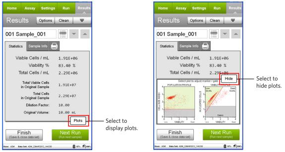
12. (Optional) If changes are needed to the cell size gate or viability marker, touch a plot to enlarge it, then adjust the cell size gate and/or viability marker as described in steps 4 and 6. You cannot adjust the nucleated cells threshold after the sample has been acquired.
