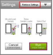
**NOTE:** If the acquisition times out (after 2 minutes), you can select **Back** to restart the adjust settings step or **Next** to accept the settings and continue to the next step. If acquisition times out, remove the
