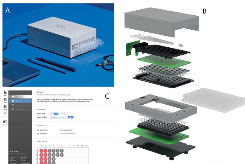
**Figure 1:** The Absorbance 96. The unique design relying on 96 individual detection units allows for a compact and maintenance-free, portable microplate reader. Open design enables plate loading. Plug-and-play functionality and power supply via USB result in maximal portability and flexibility. (A) *In-situ* appearance of the plate reader. (B) Explosion view. (C) Intuitive software interface.
