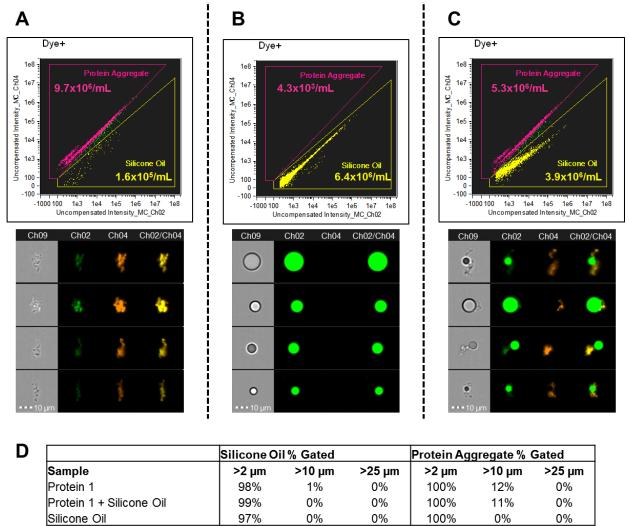
**Figure 3:** Example of FlowSight<sup>®</sup> data. Fluorescence classification of particles and representative images for (A) Protein 2 (stressed Lysozyme, 500 µg/mL), with images of aggregates, (B) Silicone Oil (0.02%), with images of silicone oil droplets, (C) a 50:50 mixture, with images of heterogeneous complexes containing both aggregate and silicone oil droplet. (D) Size distribution analysis.
